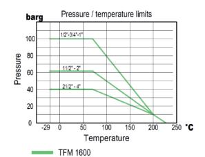
Note: Working pressure may be limited by the valve connections.
