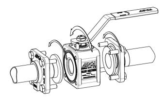
Loose body flanges make it possible to install the valve without the aligning of welded end connections. After installation the valve can rotate 360° for the desired orientation.
