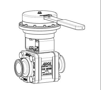
To switch the ball valve to a safe position (closed or open), as soon as the operator releases its handle.
