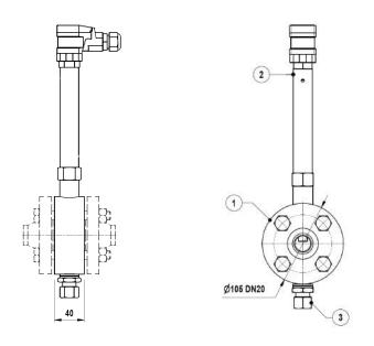
Remarks: Can be fitted into a "T" connection or into our standard chamber, providing that the probe is always in contact with the water. Any metallic parts near the probe must be at a minimum distance of 20 mm from the central end pole.
