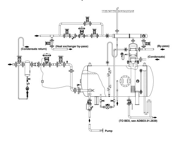
Atmospheric deaerator including ADCATherm STS series complete stainless steel heat exchanger. Make-up water crossing the heat exchanger will condense the flash steam, preventing energy waste and providing better performance for the whole system.
