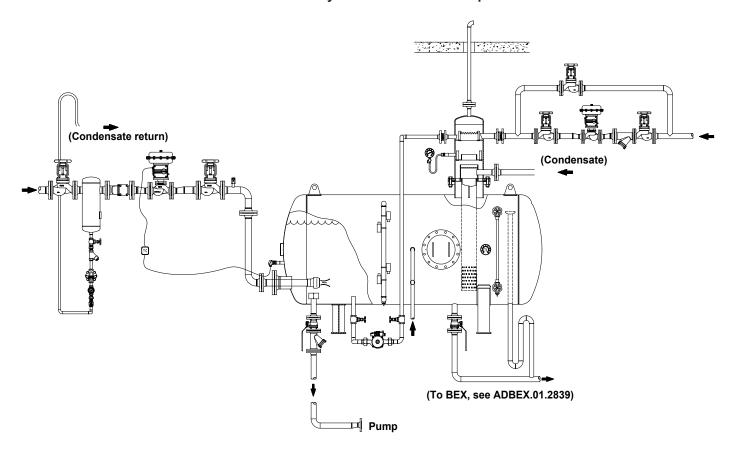
Atmospheric deaerator provides an economic system to preheat boiler feed water and remove dissolved gases.
